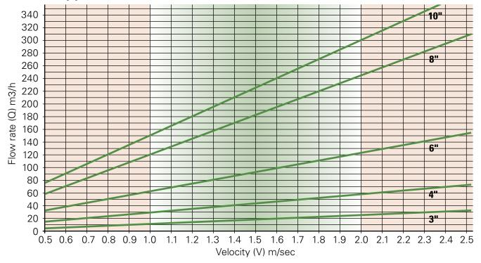
\* The graph represents the velocities in pipes of one specific standard among many. If the pipe used in the system's main, sub-main or distribution lines does not appear in the above table and graph, find the actual internal diameter of the pipe in the pipe documentation and calculate the velocity using the following formulas:
