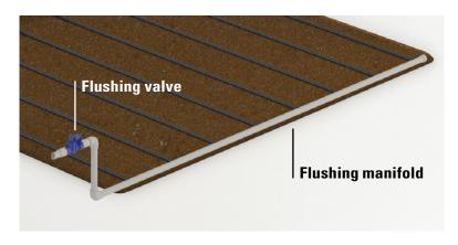
The flushing manifold is sized for a flow velocity of at least 0.5 m/sec (1.65 ft/sec) at the end of the dripperlines to ensure sediment removal.
